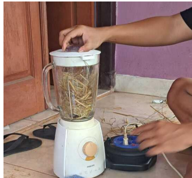
Figure 4. The process of chopping cogon grass using a blender
