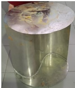
Figure 2. Savonius turbine with type of Myring n=1
